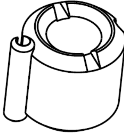
Figure 1 Threaded insert equipped with spring-type pin.
